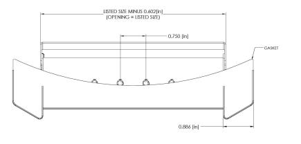
Description • Double Deflection • Adjustable Blades • Galvanized Steel Construction • Unpainted • Scoop Option Available • Made in the U.S.A
