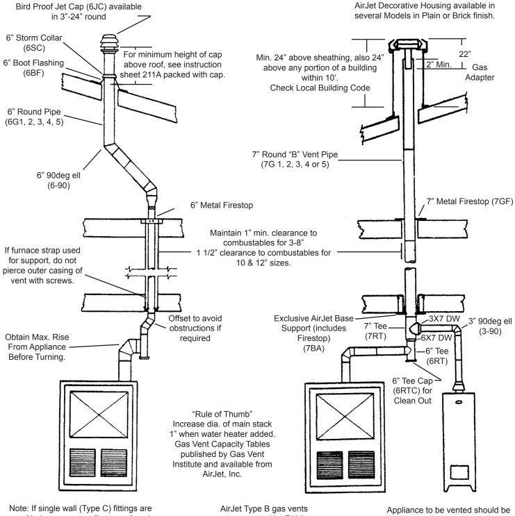
Note: If single wall (Type C) fittings are used between gas appliance and vent assembly (BA) provide 6" clearance from combustible. AirJet Type B gas vents are accepted by F.H.A and V.A. Appliance to be vented should be placed as near to vertical vent as possible.
