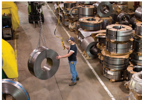
Department supervisor Cary Mejia moves a roll of steel in place to feed one of the numerous press lines.
