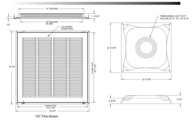
DescriptionLouvered Face, 1/3" FinsR6 Fiberglass PlenumAluminum ConstructionWhite finish
